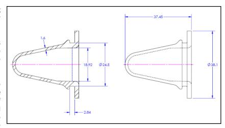
4. Our MWS units have been manufactured without the hole. This allows the end user to put the proper hole size in the MWS unit to optimize the moving wire seal.
